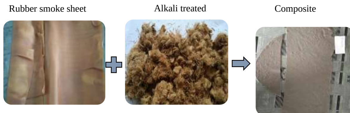
Figure 1. Preparation of alkali treated areca nut fiber-rubber composite for stopper
